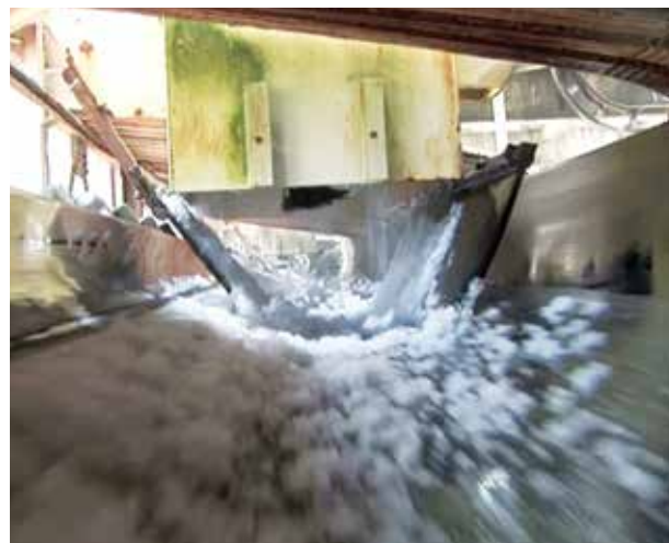
Ice at Mponeng Mine, South Africa, is pumped down into the mine to ensure a well cooled, ventilated and safe working place.
