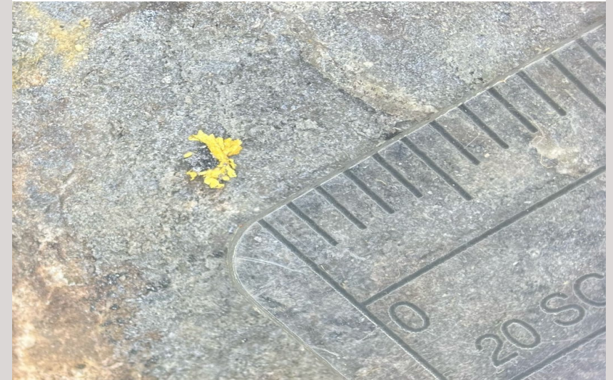
Visible gold – Merlin drill core (MER-23-0243-RD)
