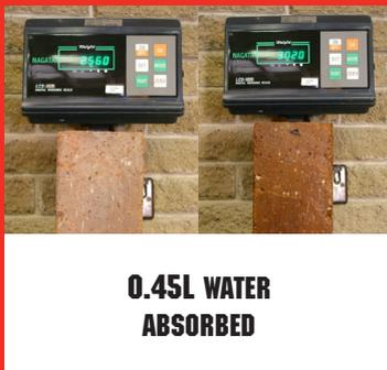
Burnt clay brick is like a solid sponge. The pictures above show the mass of the same brick dry(LHS) and wet (RHS) after 30 minutes of soaking.
