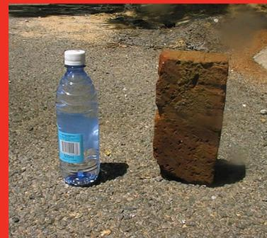
Think of each brick soaking up or “stealing” 500ml of water from the mortar.
