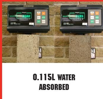
Concrete units are not as thirsty. The photos above show the same unit before and after soaking for 30 minutes.
