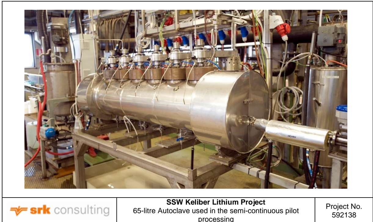
Figure 9.8: 65-litre Autoclave used in the semi-continuous pilot processing
