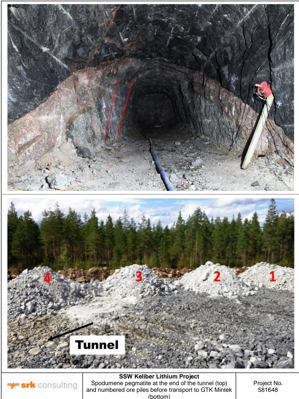
Figure 9.1: Spodumene pegmatite at the end of the tunnel and numbered ore piles before transport to GTK Mintek
