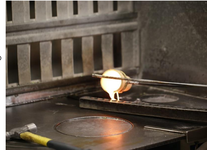
Fire Assay - US PGM recycling facility
