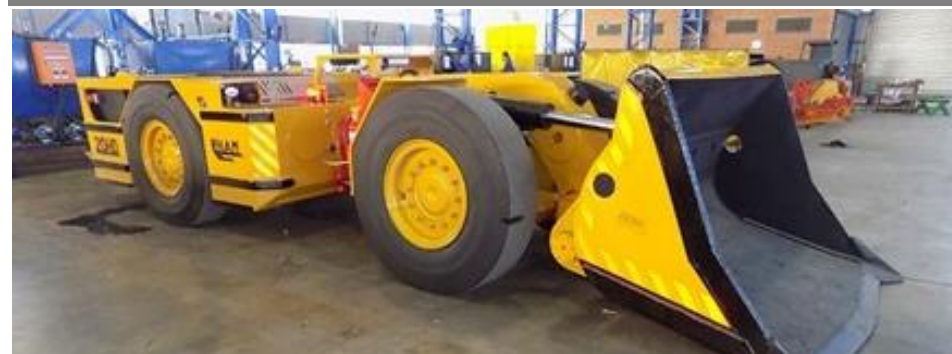
Remotely-operated battery LHD to be trialed
