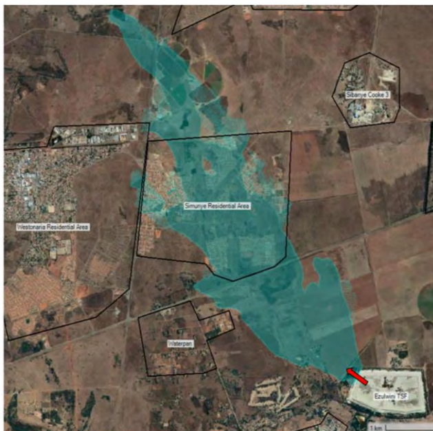
Figure 4: Inundation Map for the Rainy-day Failure at the North-Western Wall
