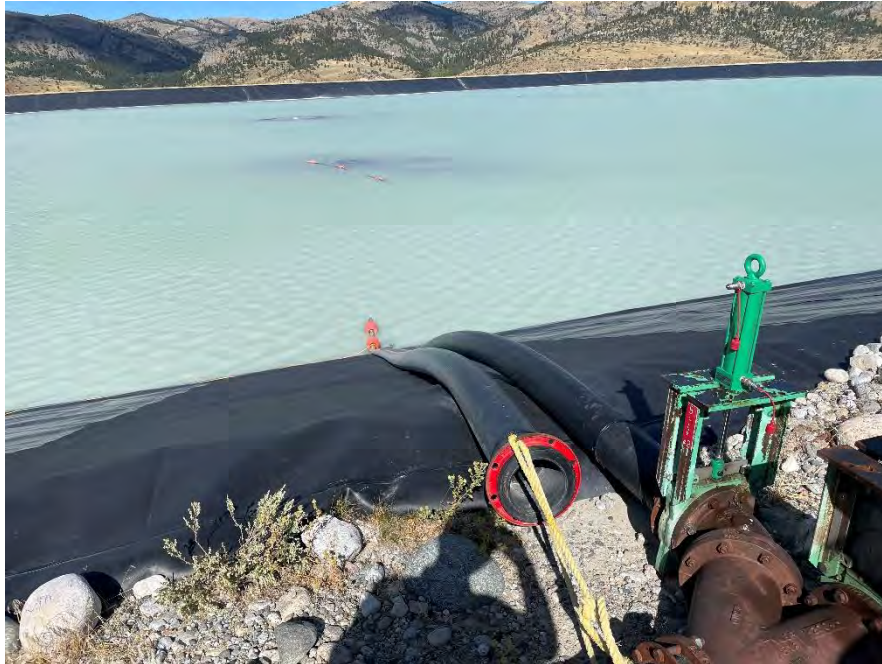
PHOTO 9 – Floating tailings discharge spigot (2022).
