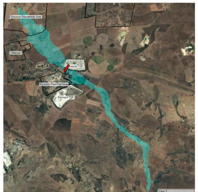
Figure 5: Inundation Map for the Rainy-day Failure at the South-Eastern Wall
