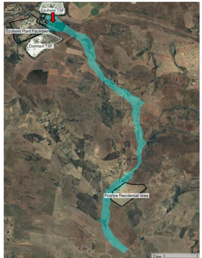
Figure 3: Inundation Map for the Rainy-day Failure at the Southern all
