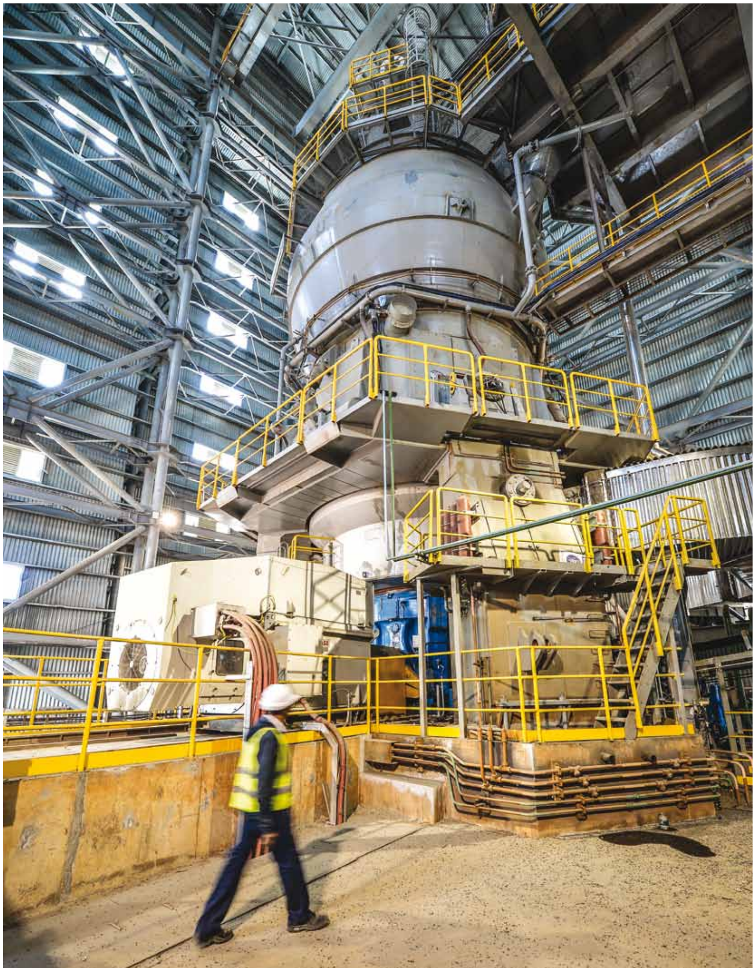
Loesche cement mill at Delmas plant capable of producing 160 tonnes per hour
