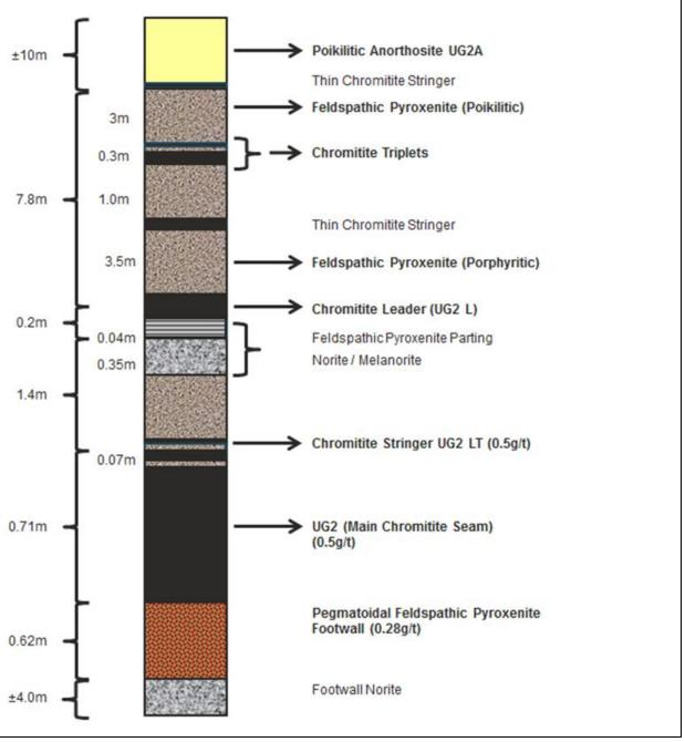
Figure 6.10 General stratigraphic column of the UG2 Reef\*
