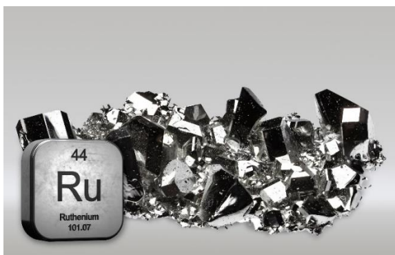
Caption: Platinum Group Metal Ruthenium shows a high catalytic activity but alone lacks stability in the operational conditions of PEM electrolysis. With the new ruthenium-iridium material class an activity boost is achieved combined with stability. (Source: Adobe Stock and Heraeus Precious Metals)
